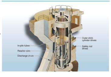
The ATR core contains a beryllium reflector to help concentrate neutrons in the core, where they are needed for experiments related to fuels and materials testing.
