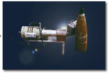
edical doctors use X-rays to see bone and tissue structure inside the body. Mechanics use computer-based diagnostic tools and borescopes to view internal engine components. And increasingly, U.S. soldiers rely on an Idaho National Laboratory (INL) technology to examine suspected chemical munitions
