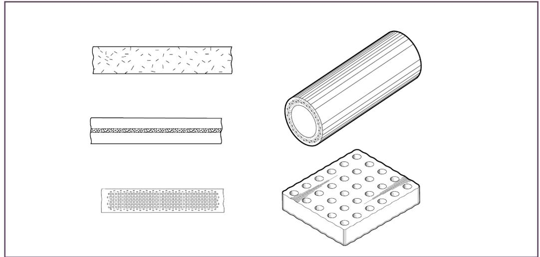
**Combustible structural composites can be configured in a variety of forms and cross-sections to best support the intended application.**
