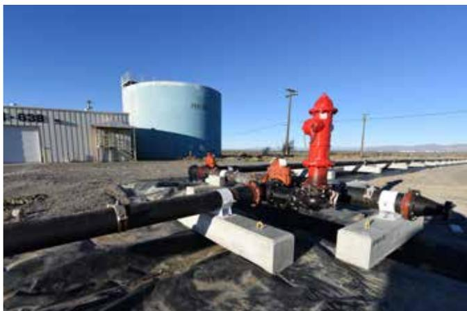
The test bed is constructed to replicate real-life conditions in a controlled environment. The cement mortar-lined iron pipe used in the WSTB is typical of the type of pipe found in U.S. cities. On the inside it may have biofilm, mineral deposits and could be corroded where the cement lining has chipped away. These factors are important because old pipe tends to absorb contaminants differently than newer pipe.
