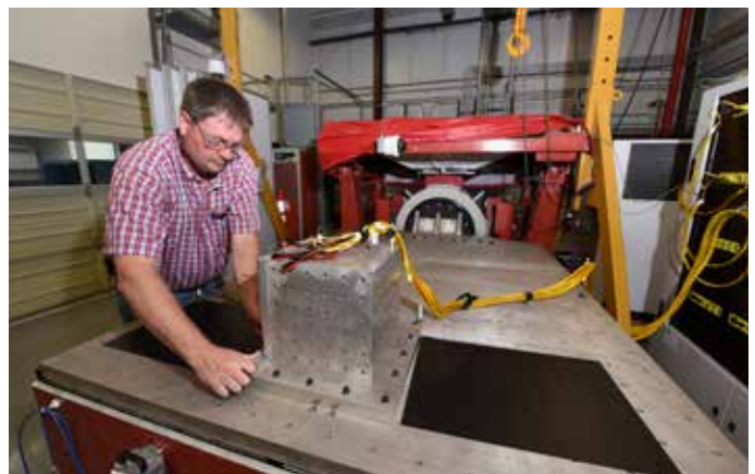
Securing a sample for testing on the Brüel & Kjær LDS V8-640 SPA56k Hydrostatic Bearing Slip Table.
