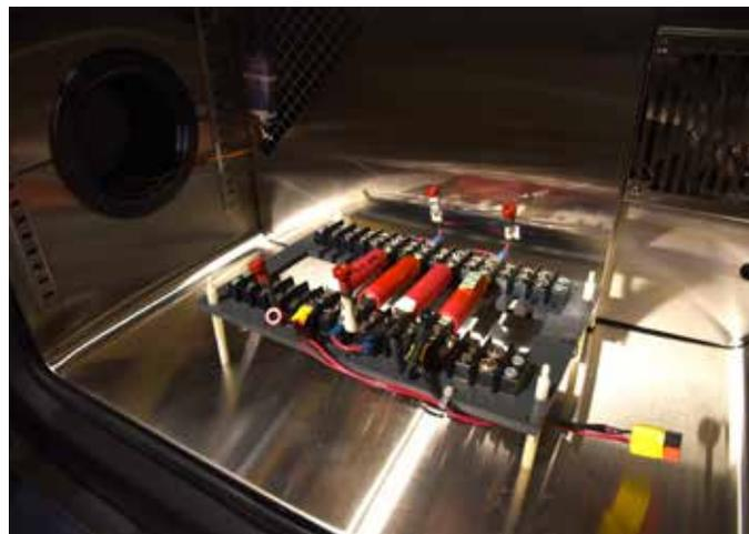
*The Impedance Measurement Box can assess a single battery cell or battery strings, which are commonly used in many consumer applications.*
