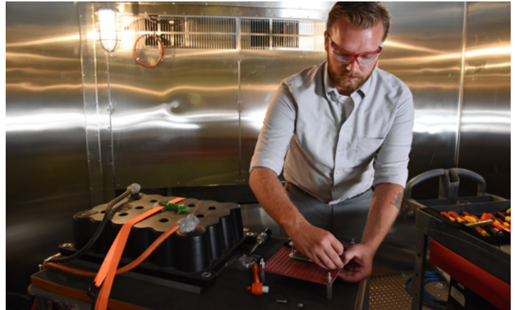
One of two walk-in chambers that allow environmental testing of vehicle battery packs in INL's Battery Test Center.
