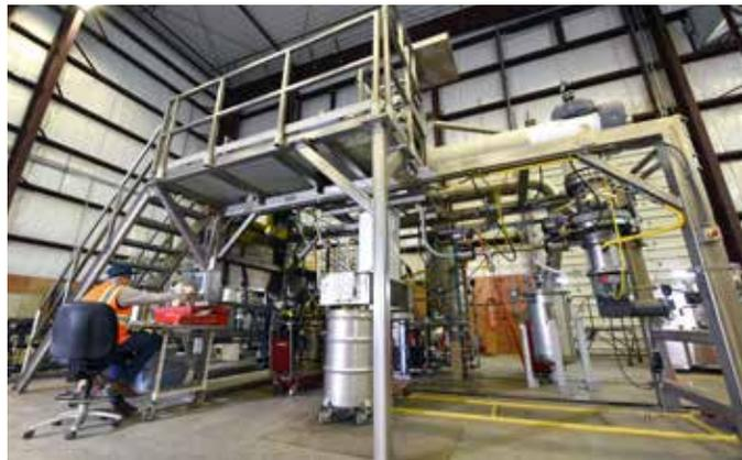
design specifications allow for dilute acid, dilute alkali, ammonia, polar and nonpolar solvents at a wide range of conditions, feedstock sizes and processing rates:
