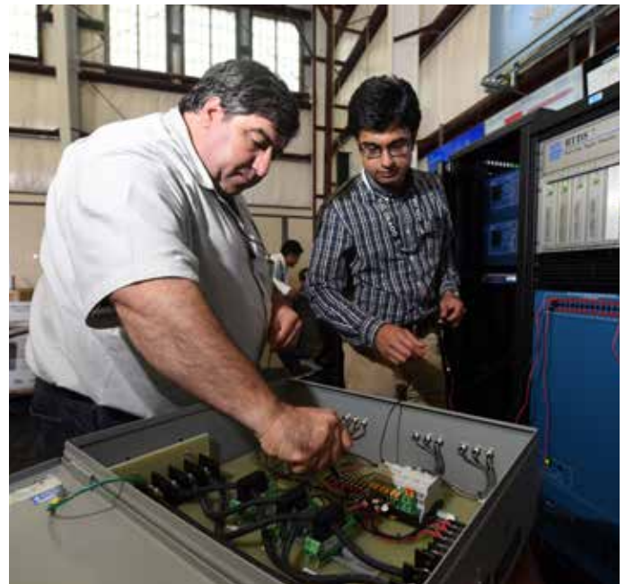
INL's Power & Energy Systems engineers use a Digital Real-Time Simulator to test hardware and controllers by emulating real-world grid events.
