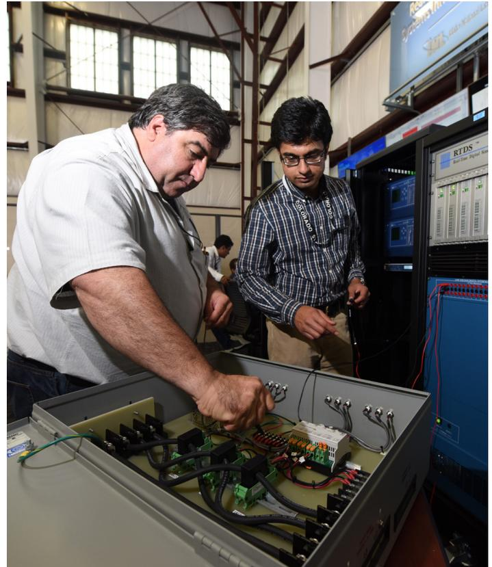
*INL's Power & Energy Systems engineers use a Digital Real-Time Simulator to test hardware and controllers by emulating real-world grid events.*
