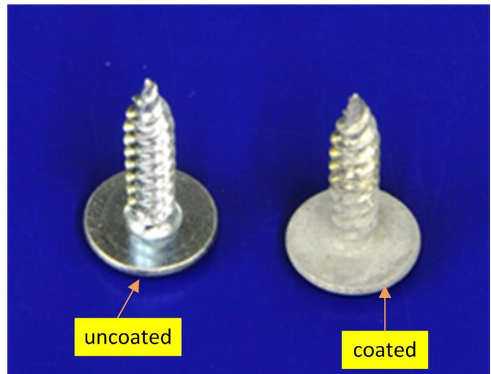
Screws before and after they are plated using bromide salts.
